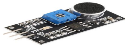
Gambar 2.5. Electric Condenser Microphone
